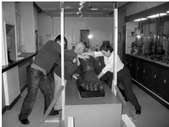
The first task was to erect a gantry, and then to tilt the foot, using brute force, in order to get the straps underneath.
